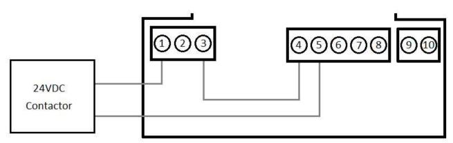
Notice the 24VDC internal power supply can't deliver large inrush currents. This is relevant when using big contactors. If the installation requires big contactors it is recommended to use AC contactors. It is also recommended to use contactors with internal transient protection.
