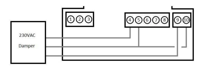
When using the AC output: notice terminal 9-10 is supplied through the same 2AT fuse as the controller. Maximum power draw is 350W.
