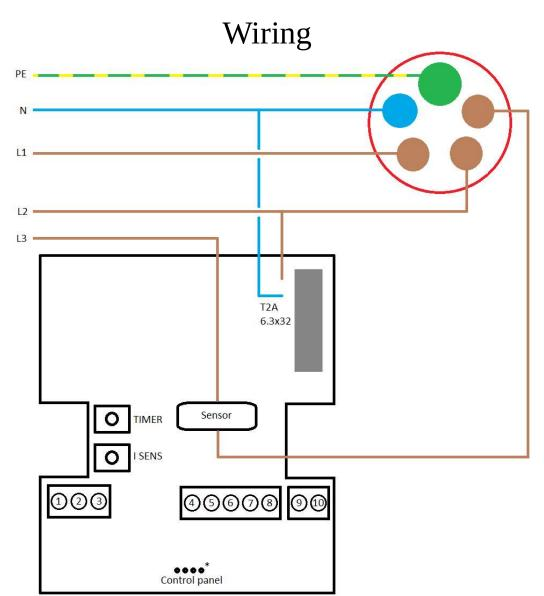
N and L are connected to the premounted wires on the controller. The conductor to be measured is looped through the sensor on the circuit board. The sensor is marked "conductor through this sensor". Notice the controller must not be powered with a conductor looping through the sensor. This can cause the controller self activate. The control panel is connected to the 4 pin header with the markings against each other. Terminal connections table below.
