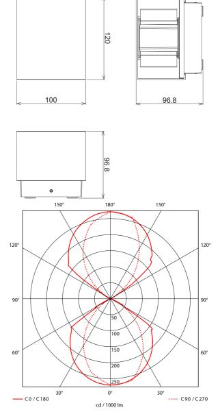
Outdoor luminaire with a modern design with up and down light. Beam angle are adjustable from 15°-210° by changing position of flaps. Made of die-cast aluminum.
