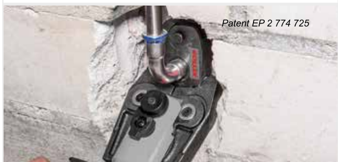
ROLLER'S pressing ring 45° (PR-2B) , with 2 pressing jaws, for applying the pressing jaws safely in places of difficult access by using an inclination of 45°.
