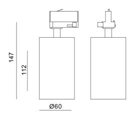
Tania Mini is a small spotlight in a contemporary design. Perfect for use at home and in other commercial settings. Choose between  ${\bf 1}$  or 3-circut connection. Front ring is sold separately. This version is with LED COB and no changeable lightbulb. L147mm Ø60mm.
