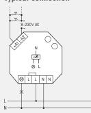
Power MOSFET up to 400 W. Energy saving lamps ESL up to 100 W. Standby loss 0.1 watt only. With adjustable minimum brightness. With switching operation for children's rooms and snooze function.
