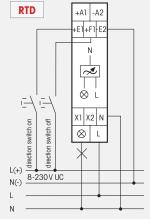
Power MOSFET up to 400 W. Energy saving lamps ESL up to 100 W and LED up to 100 W. Standby loss 0.3 watt only. With adjustable minimum brightness, maximum brightness and dimming speed. With switching operation for children's rooms and snooze function.
