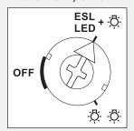
This setting must be made on the front panel on ESL and 230V LED lamps. Also with power increase with additional lamps.
