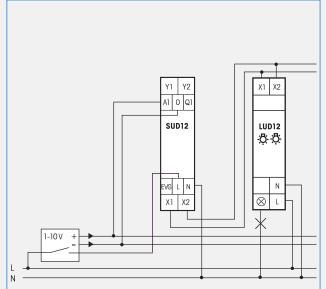
In this mode the output of a 1-10V controller can be converted at A1/O into a direct dimming function when connected to a capacity enhancer LUD12 at terminals X1/X2. The closing operation and the opening operation is also carried out externally at L of the SUD12.
