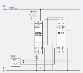
In this mode electronic ballast units and transformers with a 1-10V interface up to a total control current of 40 mA can be controlled when connected to an universal dimmer switch EUD12Z or EUD12D.
