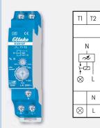
Power MOSFET up to 300 W. Energy saving lamps ESL up to 100 W. Standby loss 0.1 watt only. With adjustable minimum brightness and dimming speed. With switching operation for children's rooms and snooze function.
