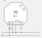
Control by pushbutton switches or light switches.
