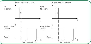
The result of combining a staircase lighting time function with an off-delay depends on how you have defined the staircase lighting time function:
