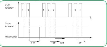
Moreover, for the off-delay, you can also select *Retriggerable and adding*. The delay time is added when the same telegram value is received, e.g. using a separate button. You can define the maximum number of additions.
