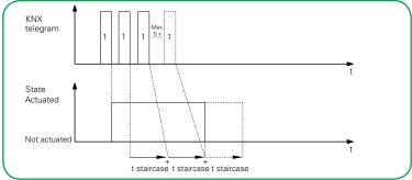
Once one or more new telegrams with the object value "1" have been received, the staircase lighting time is added to the previous staircase lighting time. The number of additions can be set. You can parameterize a maximum of 5 additions of the staircase lighting time. For example, you can add up the staircase lighting time by pressing a separate button several times.
