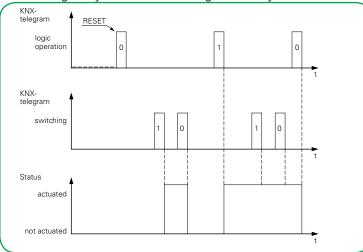
The relay can only be switched via the "switch object" if a "0" telegram has been received via the "logic object".
