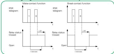
Staircase lighting time function with off-delay
