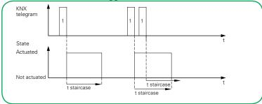
However, if the staircase lighting time is not retriggerable, the relay will switch off at exactly the moment the time elapses. If the *Manual switching off* function is activated, the staircase timer can be ended with a "0" telegram.
