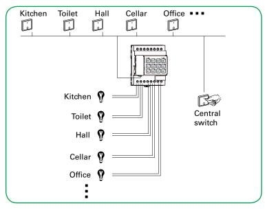
For blinds and roller shutters, there is a separate central object with a corresponding central object. In order to use the central function for the individual switch/blind/roller shutter channels, you must first enable the global function on the *General settings* tab.
