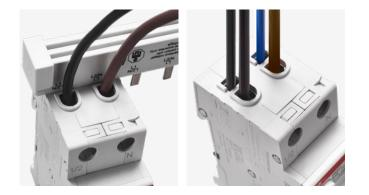
The power can be supplied parallel to the cables and busbars (either from the top or from the bottom) since the clamps consist of two different chambers: One at the front for 25 mm<sup>2</sup> busbar and one at the rear for 10 mm<sup>2</sup> phase rails or busbars.
