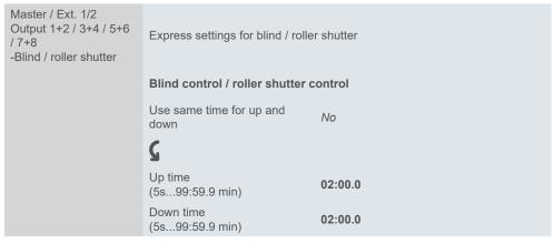
The *Running time: Up* should be parameterized slightly longer so that the end stops are always reached, even in the case of low temperatures or a heavy blind / roller shutter.
