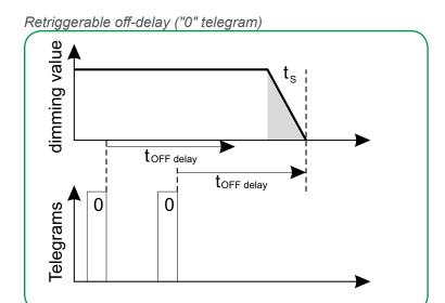
Moreover, for the off-delay, you can also select Retriggerable and adding. The delay time is added when the same telegram value is received, e.g. using a separate button. You can define the maximum number of additions.
