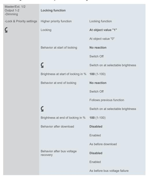
Once the locking function has been enabled, a new group object called Lock is available for the switching channel. You can activate and deactivate a channel lock using the locking object.
