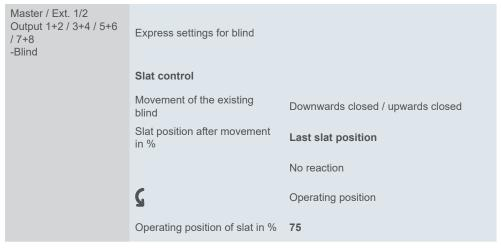
The preset value of 75% corresponds to a slat opening angle of about 45°. Since this position is set on a time-controlled basis, please refer also to the section <u>Slat</u> rotation time --> 117
