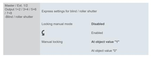
Depending on the setting, manual operation is disabled or enabled when a new telegram value is received:
