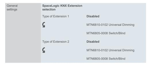
Selecting *MTN6810-0102 Universal Dimming* adds Extension 1. The 2 new dimming outputs with tabs, parameters, channels and channel functions are now available in the application.
