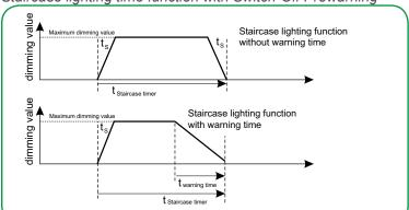
Staircase lighting time function with Switch-Off Prewarning
