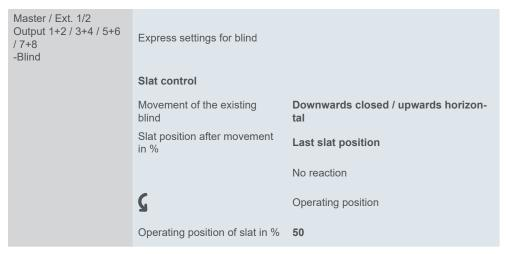
The preset value of 50% corresponds to a slat opening angle of about 45°. Since this position is set on a time-controlled basis, please refer also to the section <u>Slat rotation time --> 117</u>
