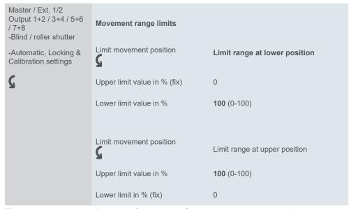
The movement range limitation function is often selected in summer when solar radiation is strong, so that it does not heat up rooms or dazzle people. The drive can no longer be moved manually all the way up, but in the event of a storm the weather alarm will move the blind to the safe position.
