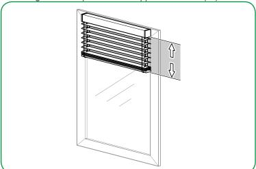
Limit range at lower position with upper limit = 0% (fix) and lower limit = 25%
