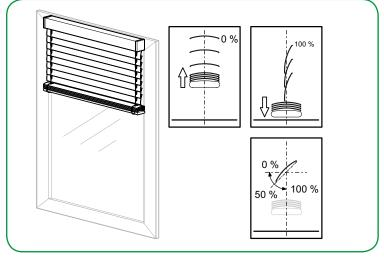
The parameter *Slat position after movement in* % allows you to define the behavior of the slats after a movement for the channel. If you set the parameter to *Operating position*, you can set an opening angle to be adopted by the slats after every downward movement.
