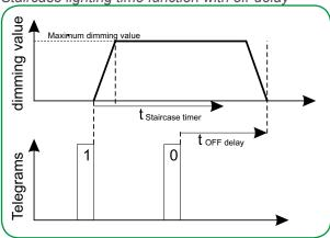
Staircase lighting time function with off-delay
