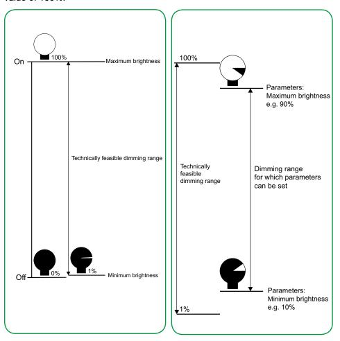
The dimming range can be limited further using the software application. This limit can be set individually for each output channel.
