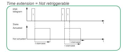
However, if the staircase lighting time is not retriggerable, the relay will switch off at exactly the moment the time elapses. If the *Manual switching off* function is activated, the staircase timer can be ended with a "0" telegram.
