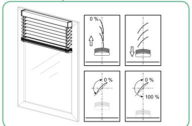
The parameter Slat position after movement in % allows you to define the behavior of the slats after a movement for the channel.
