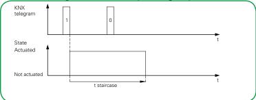
A telegram with the object value 0 has no effect. The set staircase light time continues to run normally until the end.
