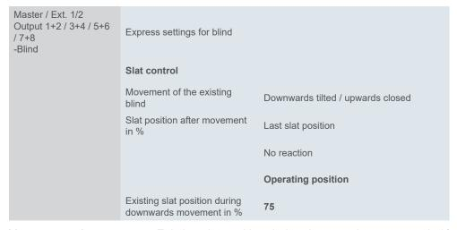
You can use the parameter Existing slat position during downwards movement in % to set the opening angle for the operating position.
