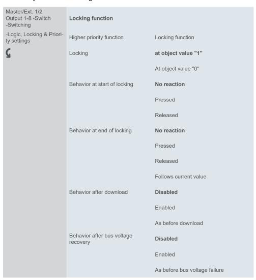
Once the locking function has been enabled, a new group object called *Lock* is available for the switching channel. You can activate and deactivate a channel lock using the *locking object*.
