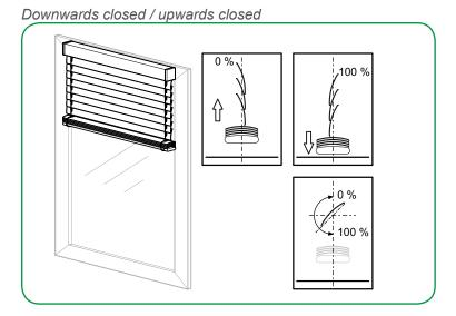
The parameter *Slat position after movement in %* allows you to define the behavior of the slats after a movement for the channel. If you set the parameter to *Operating position*, you can set an opening angle to be adopted by the slats after every downward movement.
