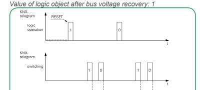
The logic object is preset with the value "1" after a RESET (bus voltage recovery and download). This enables switching to be carried out as usual using the switch object. The power-on lock is not active until a "0" telegram has been received via the logic object.
