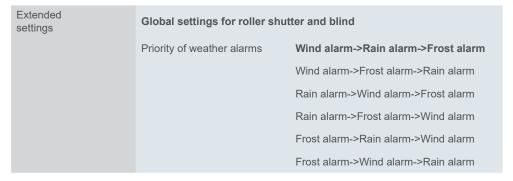
This priority setting applies to all blind and roller shutter channels for which the weather alarm function is enabled. The reactions to a weather alarm only become active if no weather alarm with a higher priority is already active. If a weather alarm is reset and another weather alarm with a lower priority is active at that time, the reactions of the alarm with the lower priority are now executed.
