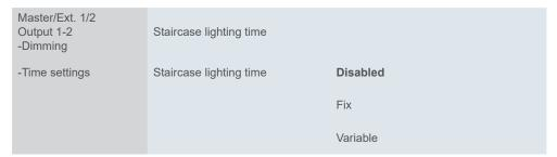
Following enabling of the corresponding staircase lighting time function, the relevant group object appears.
