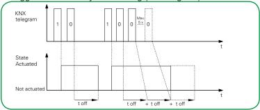
In the case of not retriggerable delays, by contrast, the relay will switch off at exactly the moment the time elapses.
