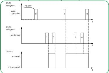
The relay can only be switched via the "switch object" if a "0" telegram has been received via the "logic object".
