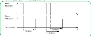
Once a new telegram with the object value "1" has been received, the staircase lighting time is restarted.
