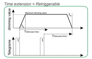
Once a new telegram with the object value "1" has been received, the staircase lighting time is restarted.
