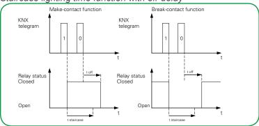
For staircase lighting time functions with *manual switching off* and warnings activated, the staircase lighting time function is immediately deactivated with a warning when an "Off" telegram is received. The off-delay elapses. No warning is generated.
