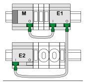
An extension cannot be put into operation if the order of the devices does not correspond to your programming in the ETS.
