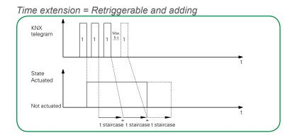
Once one or more new telegrams with the object value "1" have been received, the staircase lighting time is added to the previous staircase lighting time. The number of additions can be set. You can parameterize a maximum of 5 additions of the staircase lighting time. For example, you can add up the staircase lighting time by pressing a separate button several times.
