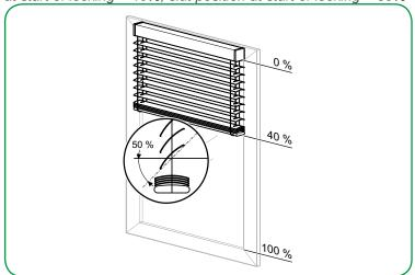
Once the drive has performed the desired action, it remains in this position and cannot be operated while the locking function is active. Only when a function with a higher priority becomes active will the reaction defined there be executed.
