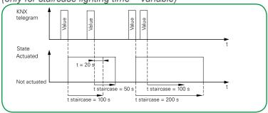
Once a new telegram has been received, the staircase lighting time is restarted with the higher value.
