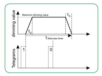
A telegram with the object value 0 has no effect. The set staircase lighting time continues to run normally until the end.
