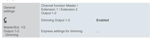
Three group objects appear for each output channel to control these basic functions.
