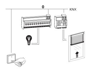
In this case, due to the fact that the roller shutter requires a certain running time to open, the light needs to be switched off with a switch-off delay so that it doesn't suddenly become dark prematurely.
