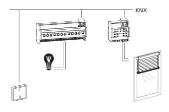
The preset function allows you, for example, to switch on the lighting and move the roller shutter at the same time by pressing one push-button. If you enter the value 0 % (roller shutter open) for preset function 1 and the value 100 % (roller shutter closed) for preset value 2, then pressing one push-button gives you the following control:
