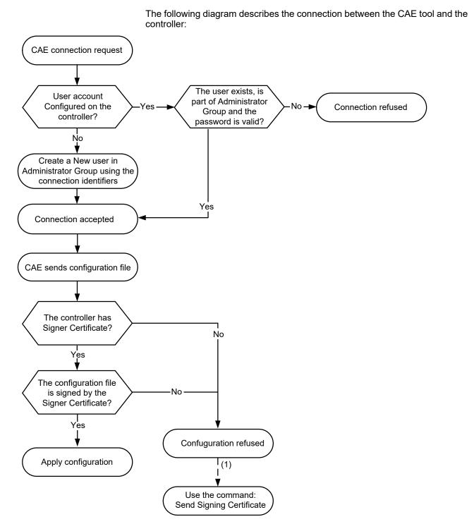
(1) In the case of the first CAE certificate has not been sent yet, use the command **Send Signing Certificate**. Subsequent operation will be proceed automatically.
