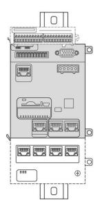
NOTE: TM3 expansion modules must be mounted above the controller.
