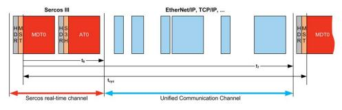
This Single Wire Architecture can be implemented using a single network cable connected to the controller. The Ethernet devices are added to the end of the cable after the Sercos devices.
