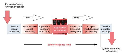
To calculate the safety response time (SRT), the system adds up the following times:
