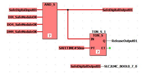
The input signal *SafeDigitalInput01* of the TM5SDI4DFS module is read and mapped via the AND\_S function to the output signal *SafeDigitalOutput01* of the TM5SDO4TFS module. Due to the AND\_S function, the *SafeModuleOK* diagnostic signals of the safety-related I/O modules are evaluated. A failure detected in any module switches the *SafeDigitalOutput01* signal off (SAFEFALSE).
