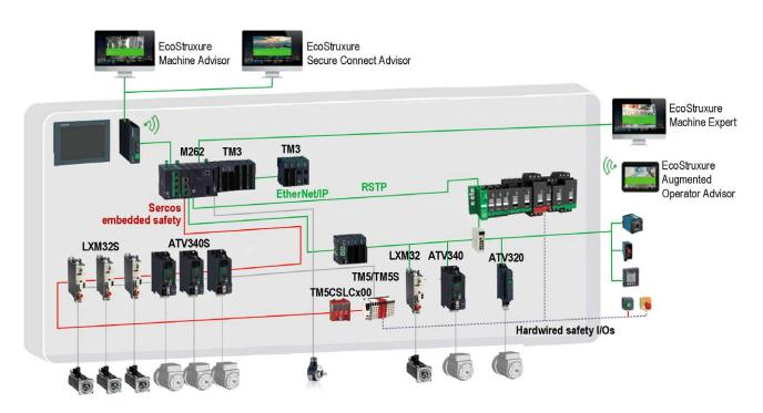
This architecture is configurable with EcoStruxure Machine Expert.
