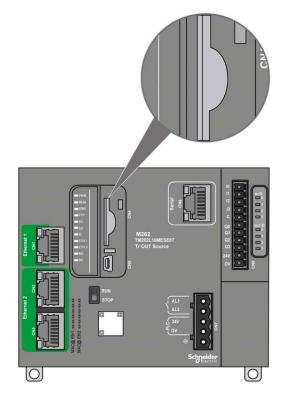
It is possible to set the Write-Control Tab to prevent write operations to the SD card. Push the tab up, as shown in the example on the right-hand side, to release the lock and enable writing to the SD card. Before using an SD card, read the manufacturer's instructions.
