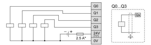
\* Use a type T fuse appropriate for the load, not to exceed 2.5 A
