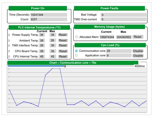
**NOTE:** The sample rate is set at 4 seconds. Setting under 4 seconds increases the **Communication core** and **CPU Load**.
