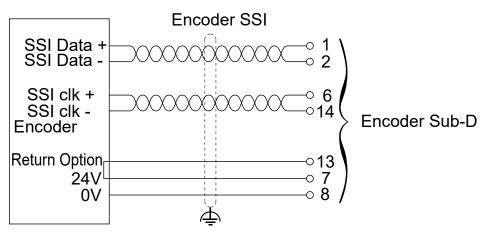
The following illustration describes the wiring diagram of an absolute (SSI) encoder (5 Vdc) mounted on the encoder interface:
