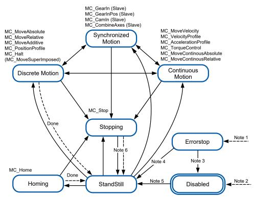
Note 1 An error has been detected (transition from any state).
