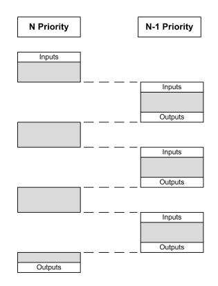
**NOTE:** If the same input is used in different tasks the input image may change during the task cycle of the lower priority task.
