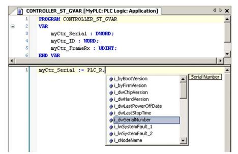
**NOTE:** In the example above, after you type the structure name *PLC\_R*, EcoStruxure Machine Expert offers a pop-up menu of possible component names/variables.
