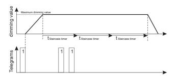
You can limit the potential running time using the "Max. number of time accumulations" parameter.
