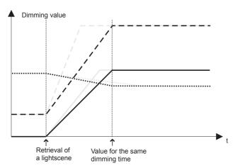
You can release the function globally for the device via a parameter, and set the corresponding dimming time after release:
