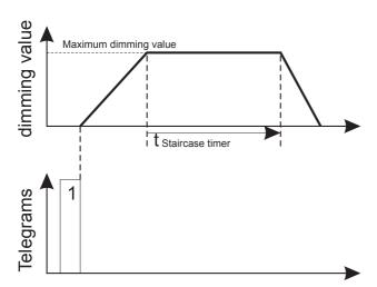
You can activate the staircase lighting function for a channel via a parameter:
