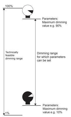
The parameterisable dimming range is set using the following parameters:
