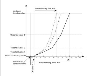
The ON delay is also retained even with a "same dimming time". The dimming curve is compressed or extended in such a way that the dimming value is reached after the same dimming time. In other words, calculation of the new dimming curve takes into account the pure dimming time (the same dimming time minus ON delay time).
