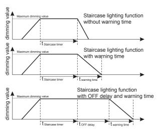
Regardless of which dimming value the output has after the staircase lighting function has expired, the time duration for the dimming-down procedure always corresponds to the warning time when the cut-out warning is active.
