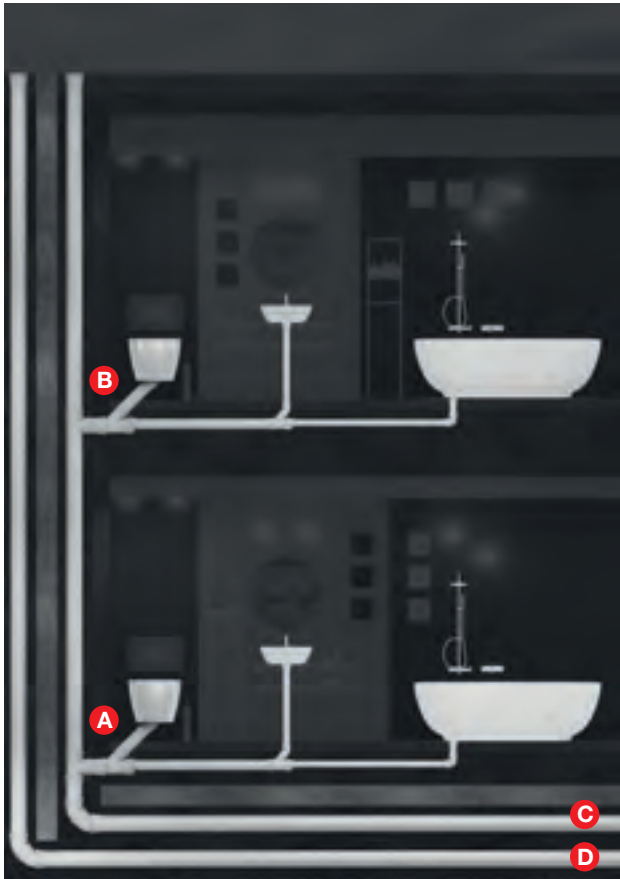
Fig. 11: Minimum fall for waste water pipes, example.
