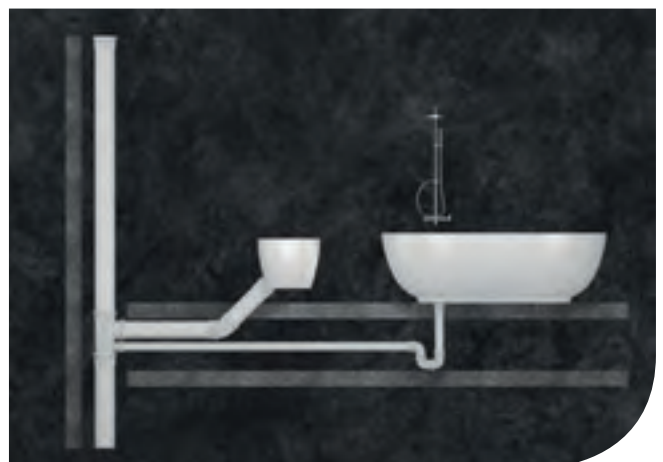
Fig. 16: Correct entry into a downpipe.
