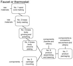
No. 1: The sand core for the base body is made. No. 2: The body of the faucet is cast from brass using the sand core.
